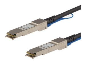
The QSFPH40GCU5M is a Cisco QSFP-H40G-CU5M compatible direct-attach copper QSFP+ cable that's designed, programmed and tested to work with Cisco brand compatible switches and routers and complies with MSA industry standards.
